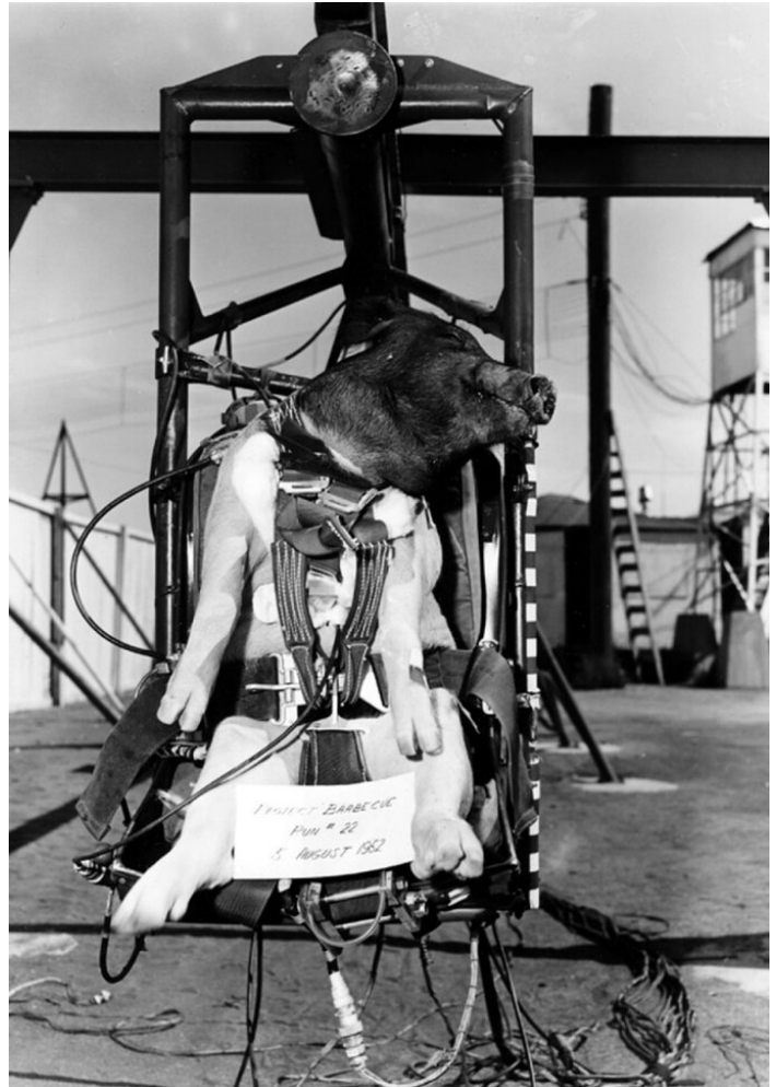
Hogs were used in crash applications in both the aviation and automobile industries. The sign "Project Barbecue, Run #22, 5 August 1952" referred to the fact that—following investigative autopsies—these nonhuman cosmonauts were cooked and eaten. Photo: USAF, Courtesy New Mexico Museum of Space History.
